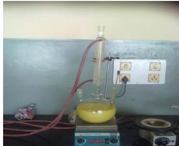
Fig. 7 Magnetic stirrer used for transesterification
