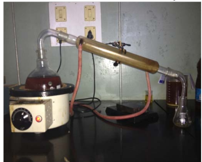
Fig. 8Methanol recovery through distillation
